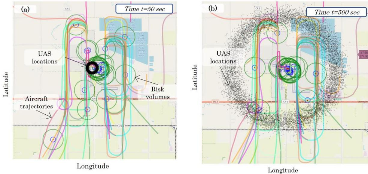
Figure 18. Probabilities of MAC, NMAC, and WC at when the (a) UA failure occurred at '0' seconds (b) Peak probabilities when UA failure occurred at different times.
