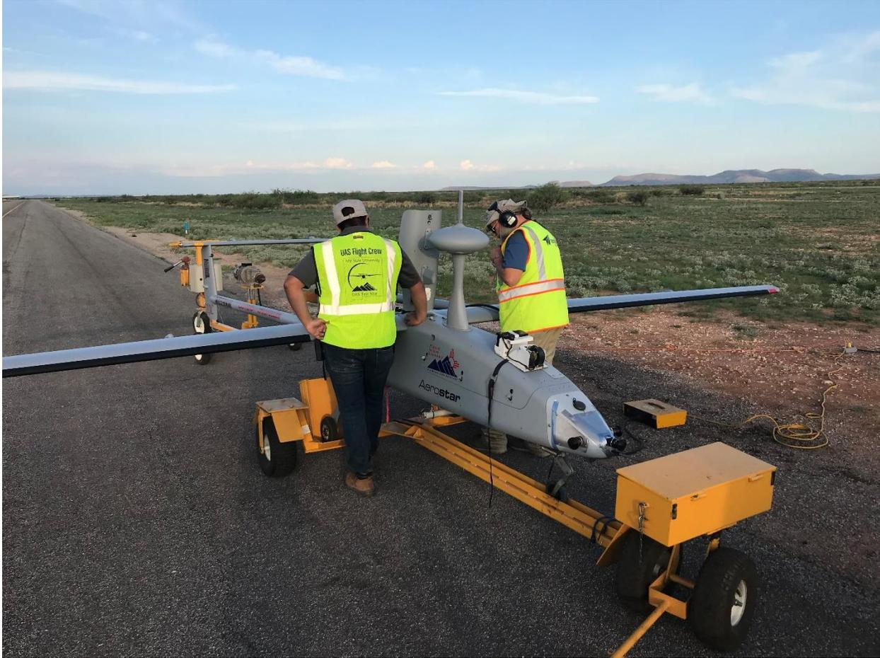
Figure 9. Aerostar undergoing pre-flight checks before transport to the flight line.
