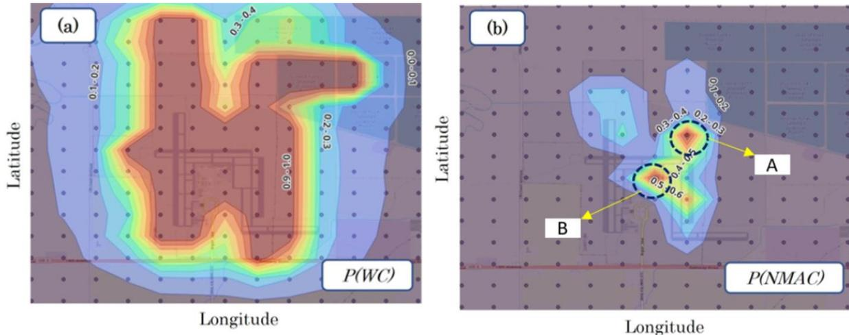
Figure 20. Risk probability dependence on the UAS failure location simulated in scenario-III (a) risk probability associated with well-clearance (b) risk probability associated with NMAC.
