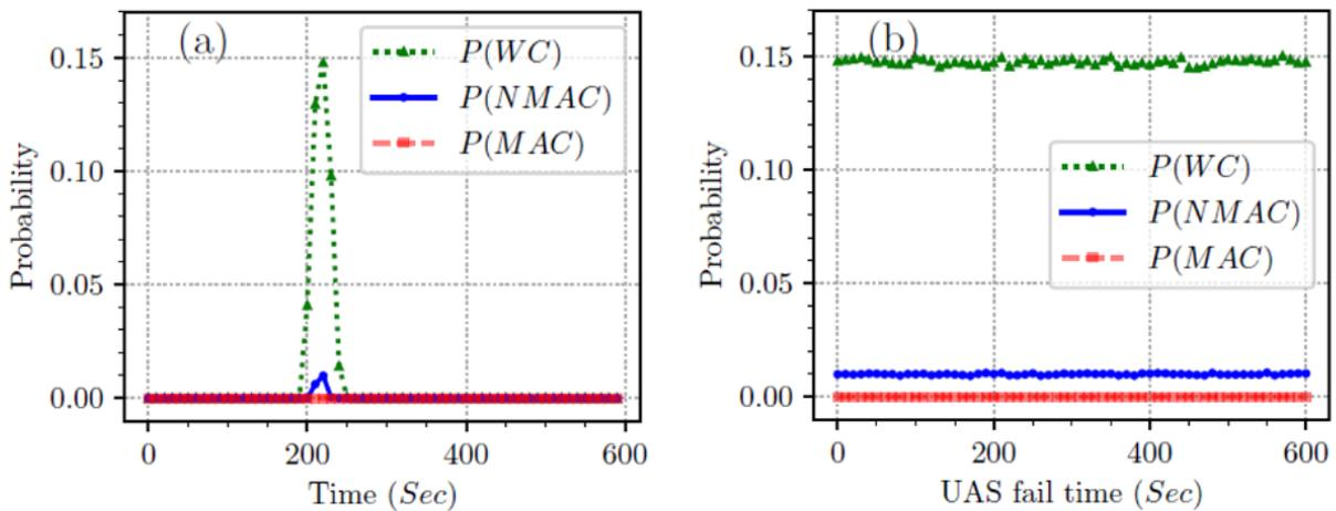
Figure 16. Probabilities of MAC, NMAC, and WC at when the (a) UA failure occurred at '0' seconds (b) Peak probabilities when UAS failure occurred at different times.
