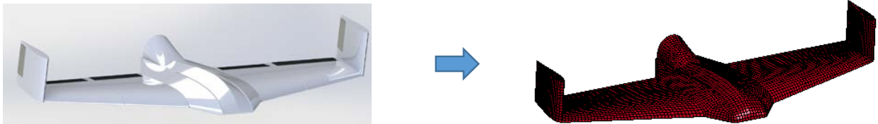
Figure 53 - (Left) CAD model and (Right) FE Model for a Fixed Wing UAS GZ500
