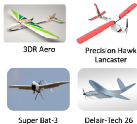
Figure D - 4 - Fixed Wing UAS with Standard Configuration
