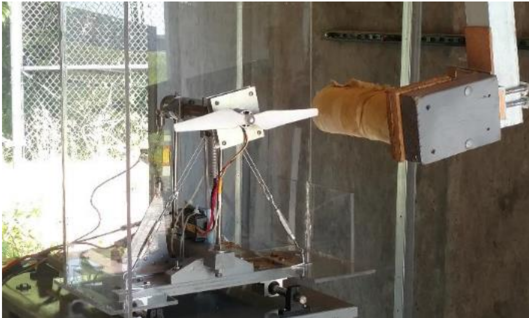
Figure 28 – Laceration Testing Setup
