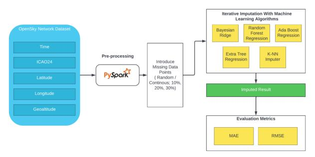
Figure 29. Overview of ML framework for Imputing Missing Data for ADS-B and GPS Dropout.
