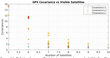
Figure 64. Relation between Positioning uncertainty and visible Satellites
