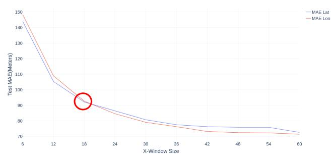
Figure 33. MAE in meters Lat and Lon, kNN Regressor.
