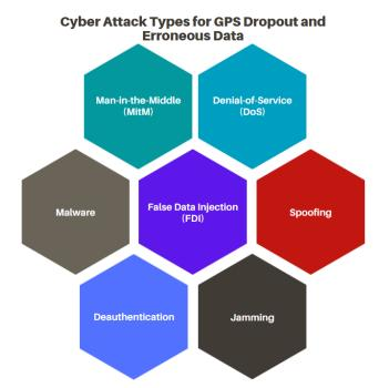
Figure 11. Cyber-attacks that compromise the availability and integrity of UAV GPS data.
