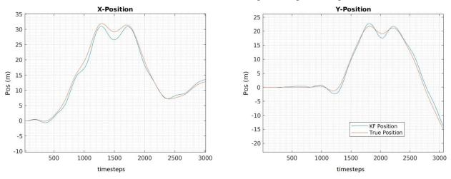
Figure 70. Position Estimation integrating OF Velocity Measurements.
