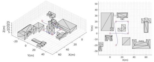
Figure 49 .UAV Reference Trajectory and Waypoints.
