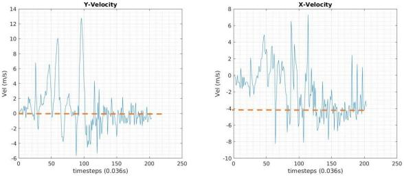
Figure 73. Velocity Measurements by only Optical Flow Odometry in real Data.
