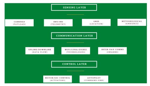
Figure 10. Operating framework for a UAS.
