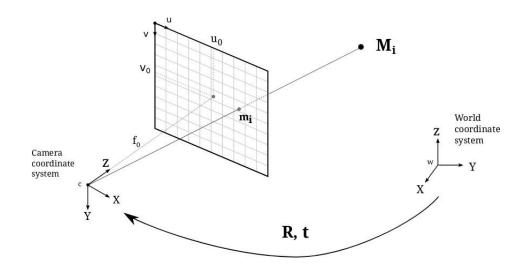
Figure 55. Pinhole Camera Model.
