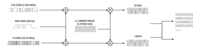
Figure 44. Illustration of the Generation of I/Q binary data using C/A and P codes.
