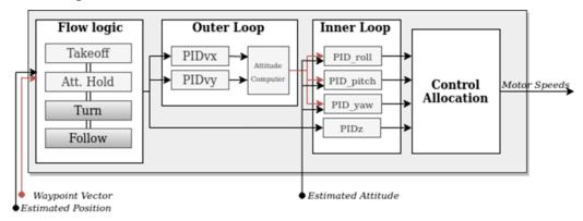
Figure 52. Position Control Scheme with Fuzzy velocity referencing.
