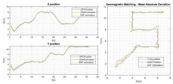
Figure 75. Trajectory S - Geomagnetic Matching Position estimation.
