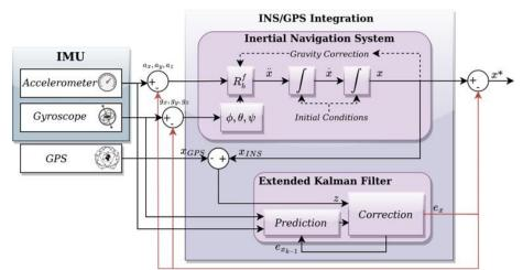
Figure 50. INS-GNSS loosely coupled integration.
