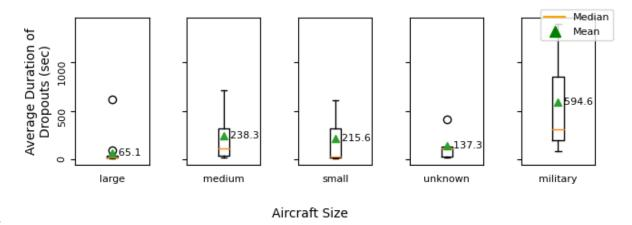
Figure 18. Effect of the aircraft size on the average dropout duration.
