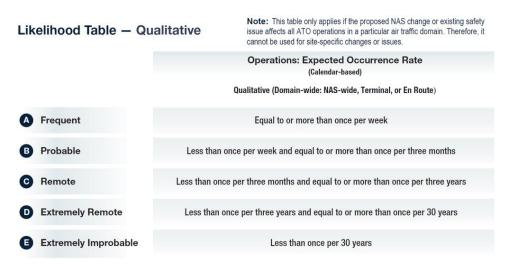
Figure 5. Qualitative Likelihood Table for Unmanned Aircraft Systems from the Safety Management System ATO SMS Manual.
