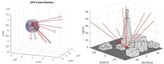
Figure 47. GNSS Signal Modeling for Shadowing Multipath Effects.
