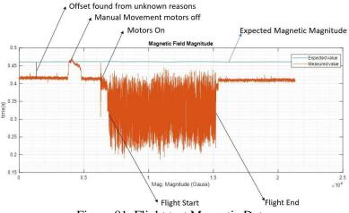
Figure 81. Flight test Magnetic Data.
