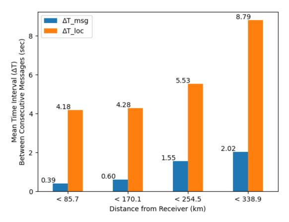
Figure 22. Distance from Receiver vs mean time interval between messages.
