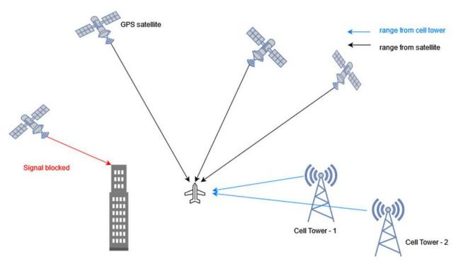
Figure 36. Conceptual diagram of cell towers augmenting GNSS positioning of an aircraft when a satellite signal is blocked.
