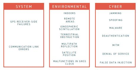
Figure 7. Categorization for causes of dropped and erroneous GPS data.
