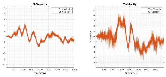
Figure 68. Velocity Measurements by only Optical Flow Odometry.
