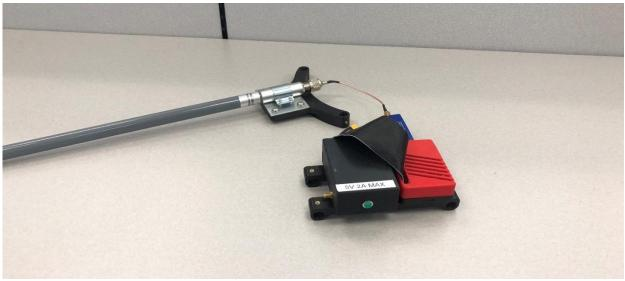
Figure 12. ADS-B Logger Payload.
