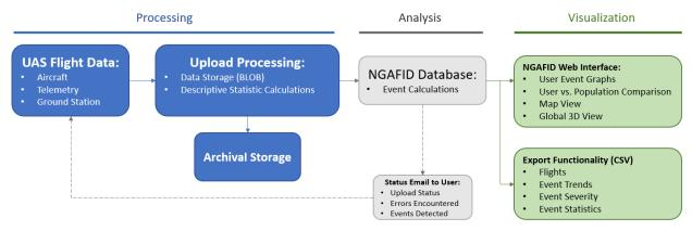
Figure 8. NGAFID Data Flow Diagram.
