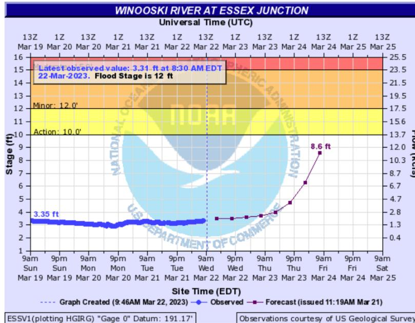
Figure 2. Hydrograph observation and forecast for Winooski River between March 10-25, 2023.
