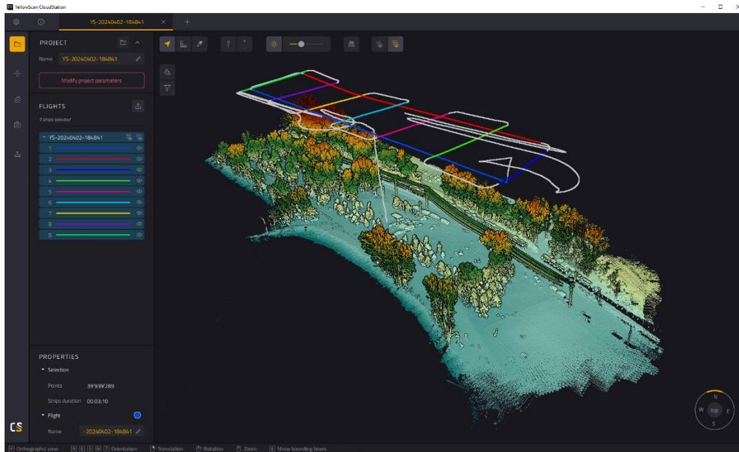
Figure 75. Intermediate step of LiDAR data processing in YellowScan Cloudstation software, displaying flight lines above and initial point cloud below.
