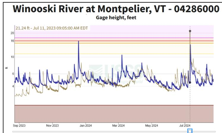
Figure 21. Winooski River guage height exceeding record flood stage at 21.24ft at 0900 EDT on July 11, 2023.
