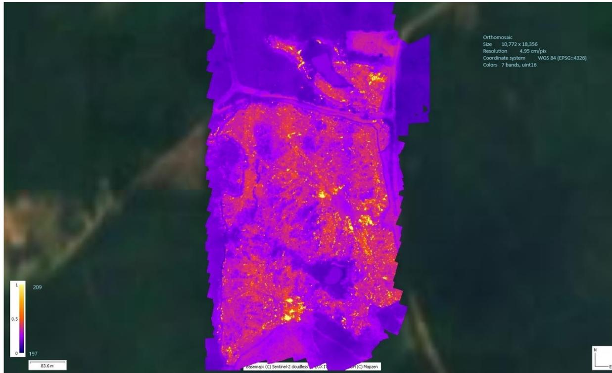
Figure 122. Altum thermal composite image the day after the burn showing many active hot spots.
