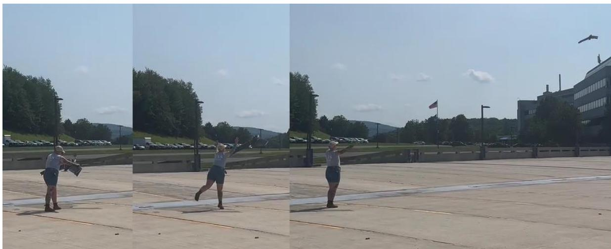
Figure 27. Sequence of eBee X launch by PIC. Note that the PIC had temporarily removed their high-visibility vest identifying them as a UAS PIC for the launch sequence, due to safety concerns with loose fitting fabric and the rear UAS propeller.
