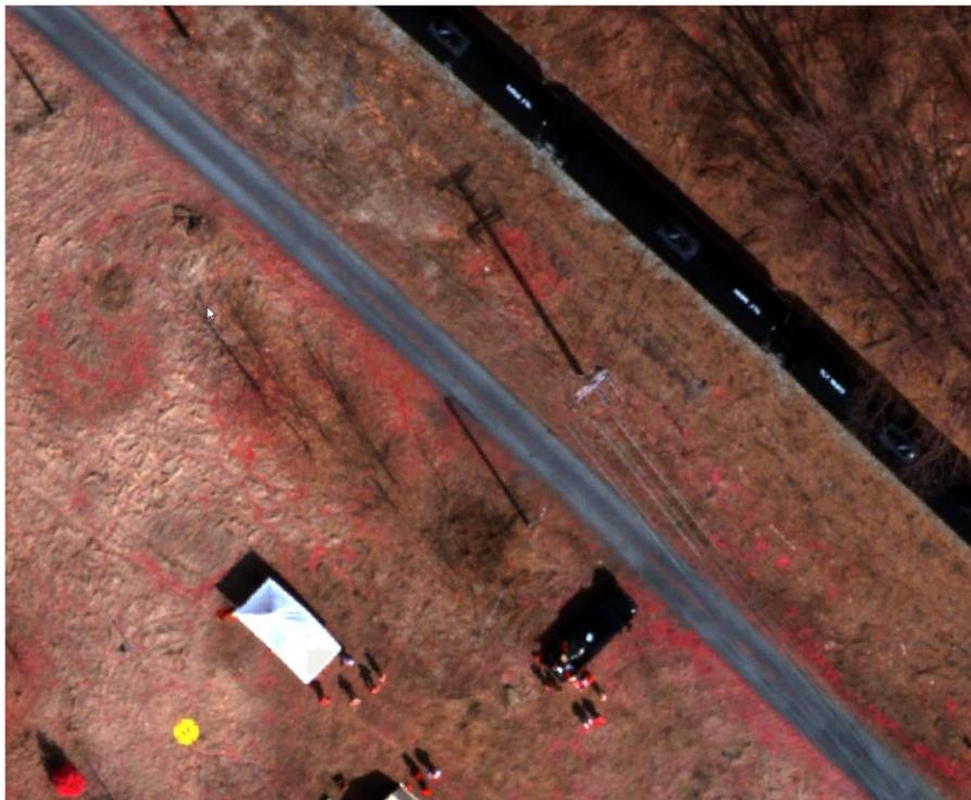
Figure 73. Multispectral orthoimagery displayed as false-color composite (NIR as red color gun).
