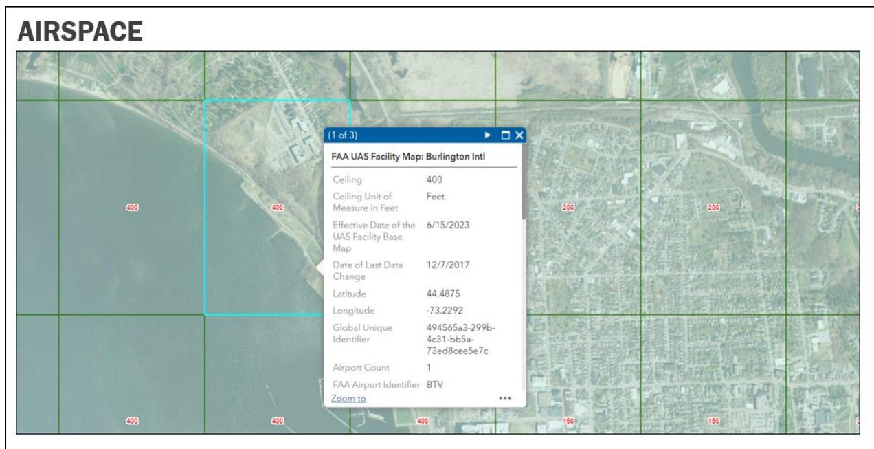
Figure 18. The LAANC cell for the site is selected, revealing a ceiling height of 400ft.
