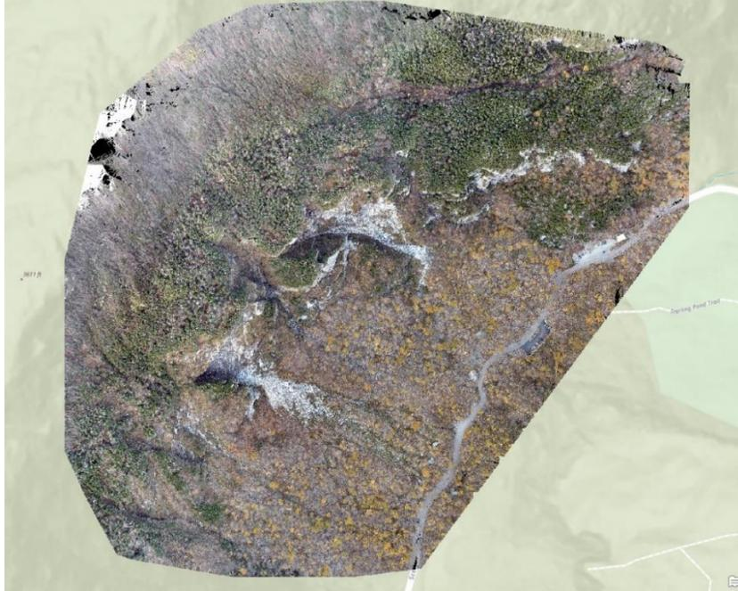
Figure 48. The true-color orthomosaic generated from processing the two UAS mapping imagery collections together.
