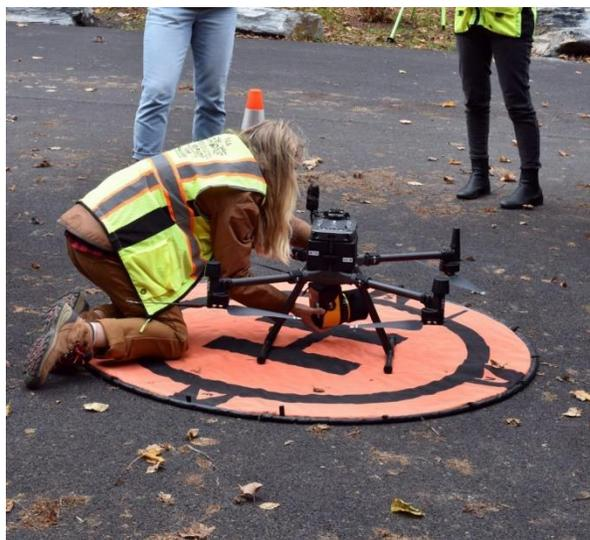
Figure 45. RPIC prepares LiDAR sensor for data collection.
