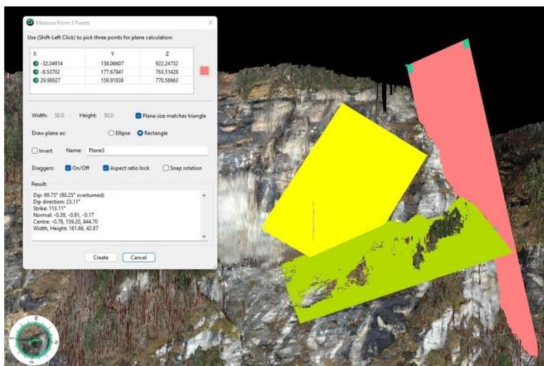
Figure 52. Oblique view of photo-textured point cloud collected using sUAS at Smugglers Notch. Image shows how the georeferenced 3D data can be used to accurately measure features that cause rock falls at the site. Three fracture sets (colored planes) intersect to form a large hazardous region (arrow) that is likely to collapse in the future. Image and geological analysis by Keith Klepeis using LIME software.
