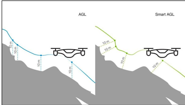
Figure 42. Illustration of UgCS Smart AGL flight planning capabilities in steep terrain. (Image: SPHEngineering).
