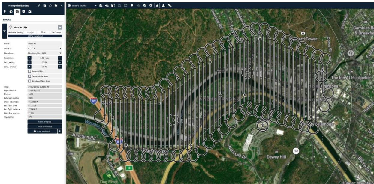
Figure 26. eBee X mapping flight plan for area of interest displayed in eMotion 3 software.
