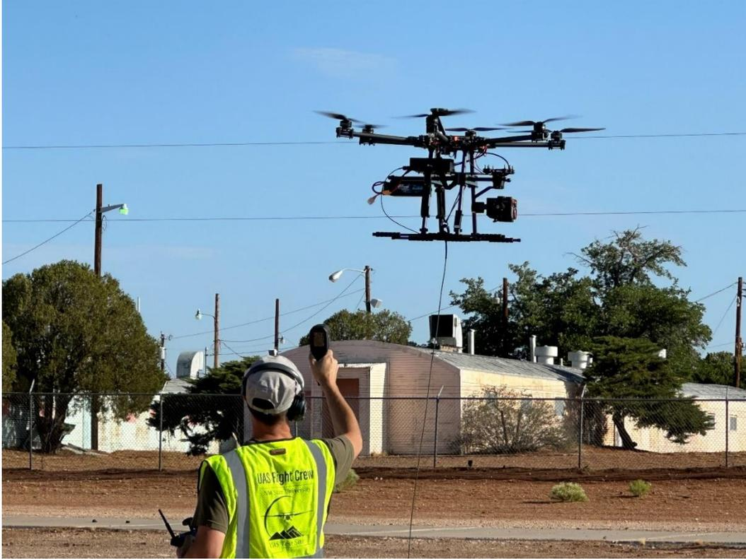
Figure 78. Component temperature measurement in flight using hand held FLIR.
