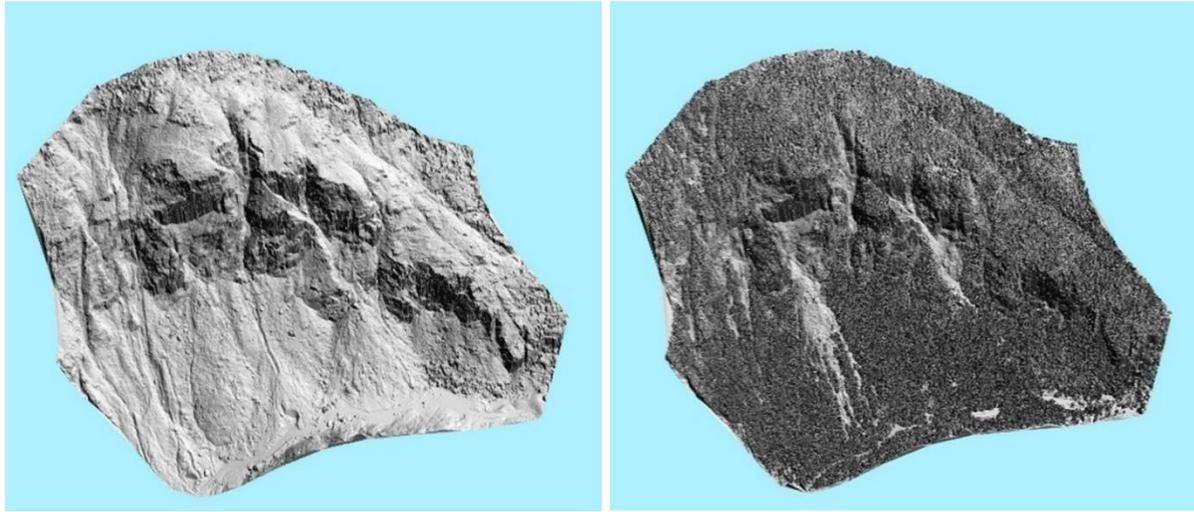
Figure 50. DEM (left) showing only bare earth, and DSM (right) showing bare earth and above-ground surfaces.
