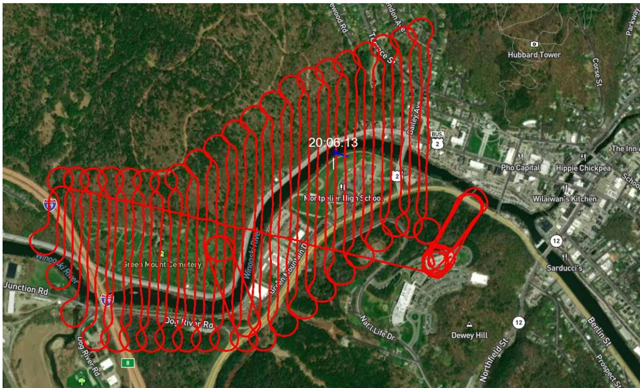
Figure 28. Trajectory of first eBee X flight from 15:25 to 16:24 EDT.
