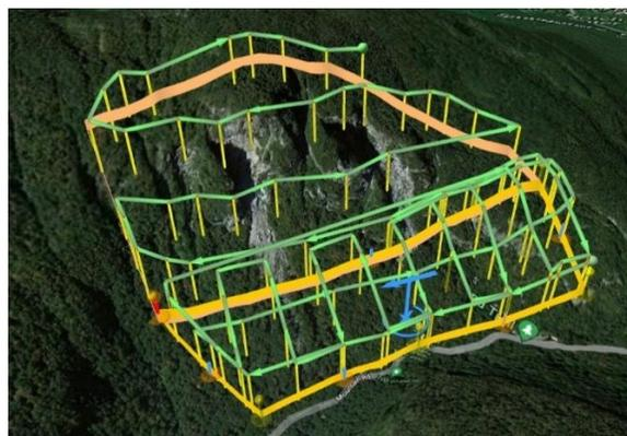
Figure 43. The LiDAR flight area is outlined by the yellow polygons, with the green lines representing the path of the UAS.
