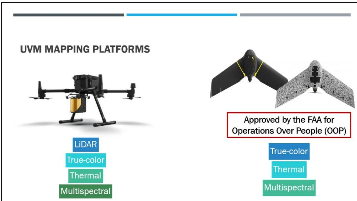
Figure 11. UVM platform options and capabilities for mapping.
