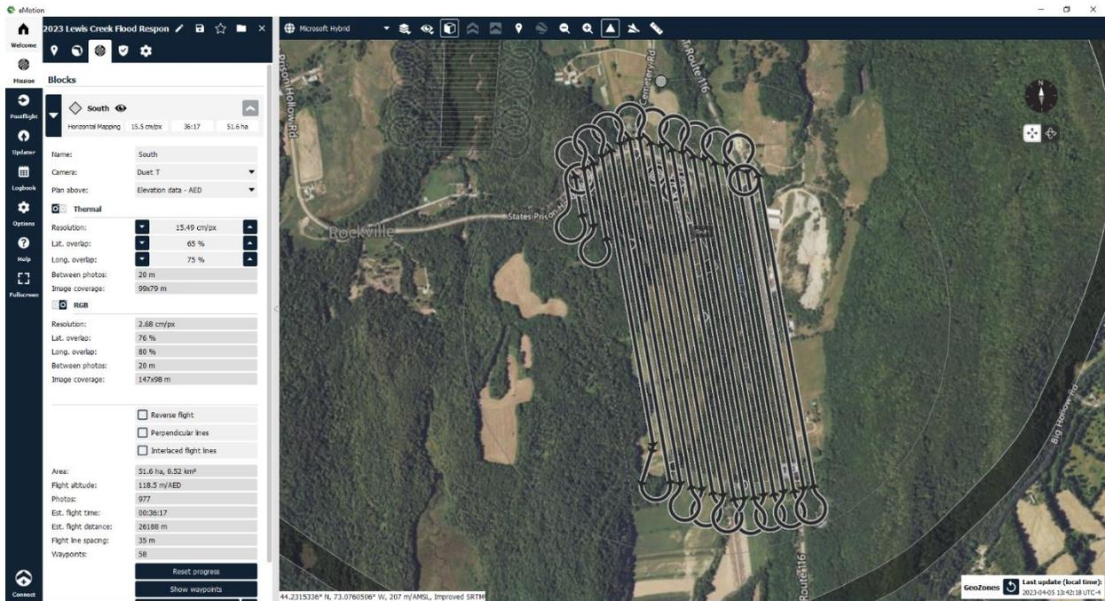
Figure 3. eBee X mapping flight plan.
